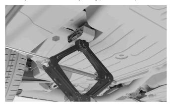
g Raise the car to an appropriate height. Do not raise it higher than what's necessary for the work you're doing.
