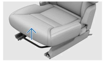
Grasp and pull the handle under the seat cushion upwards.
