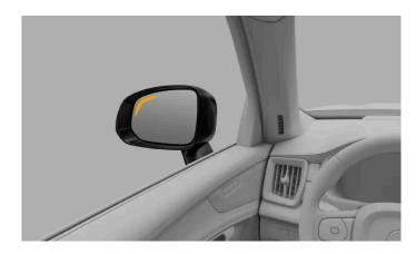
When a vehicle is detected in or approaching your blind spot, a light appears in the wing mirror.
