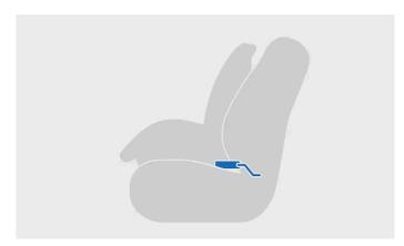
Child restraint installed using ISOFIX
