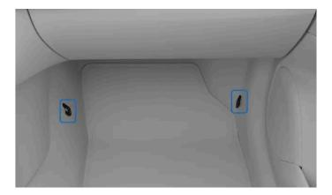
The lower tether anchorage points for the front passenger seat are located on the sides of the seat's footwell.
