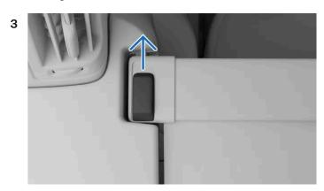
There are lock buttons at the ends of the load cover. Push the button on one side forwards and hold it in place while lifting the end of the load cover. Do this for the other end of the load cover as well.
