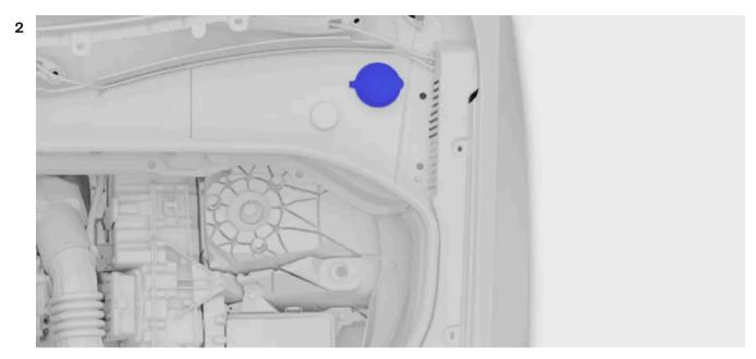
Locate the blue cap with the washer fluid symbol and open it.
