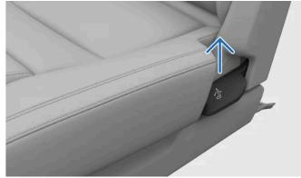
Pull and hold the handle on the side of the seat upwards to unlock backrest movement.
