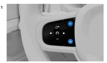
Adjust the time interval to vehicles ahead using the buttons on the steering wheel.
