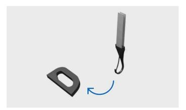
Fastening tether to lower tether anchorage point
