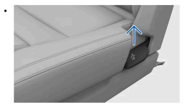
Pull the handle on the side of the seat upwards.
