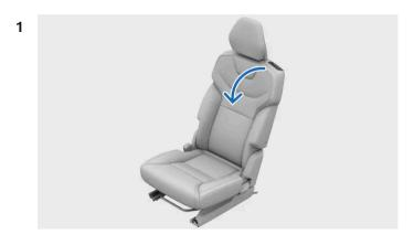
Pull the handle on the top of the outer seat backrest.
