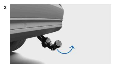
Manually pull the towbar to its end position.
