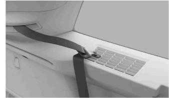
Keep the third row seatbelt out of the way when using the load cover. Pull the seatbelt back and hang it on the belt knob.
