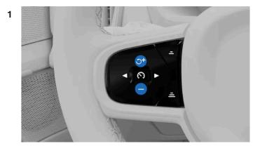
Adjust the target speed using the buttons on the steering wheel.
