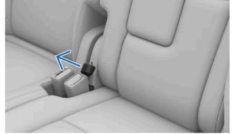
Pull and hold the strap on the side of the seat to unlock backrest movement.
