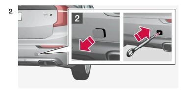
Remove the cover – press on the marking with a finger while you fold out the opposite side/corner.
