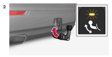
Lock the towbar by moving it back to its retracted position, where it is locked.
