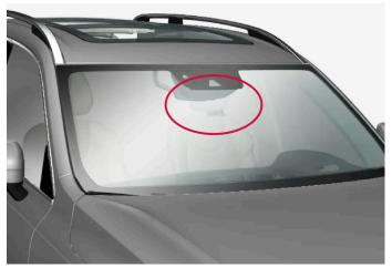
Location of front camera and radar unit
