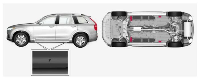
The triangles in the plastic cover indicate the locations of the lifting points (marked in red).
