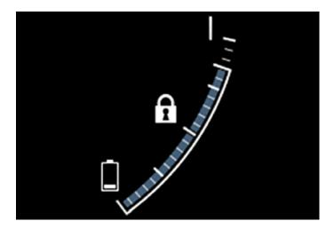
The symbol **f** is shown in the hybrid battery gauge when Hold is activated.
