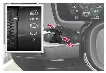
Steering wheel stalk switch with rotating ring.
