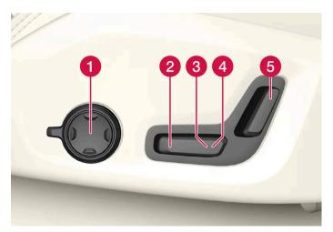
The illustration shows the controls from a car with four-way lumbar support\*. Cars with two-way lumbar support\* do not have the rotatable multifunction control.
