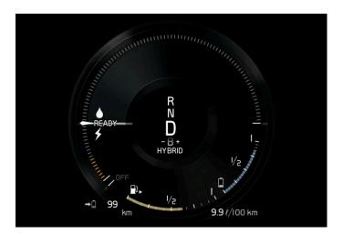
The hybrid gauge shows in different ways the relationship between how much power is being taken from the electric motor and how much power is available.
