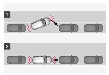
Principle for positioning during parallel parking.
