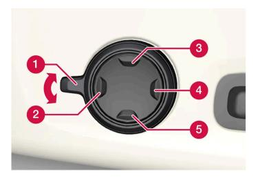
1 Activate the multi-function control by turning the control 1 upwards/downwards. The seat settings view will be shown in the centre display.
