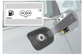
Choose fuel that is approved for use in the car in accordance with the identifier [1] on the inside of the fuel filler flap. See information on approved fuels and identifier in the section on "Petrol".
