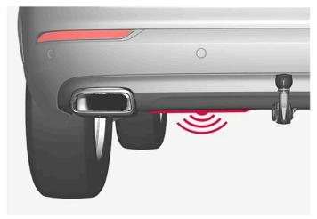
The sensor is located on left of centre in the bumper<sup>[1]</sup>.
