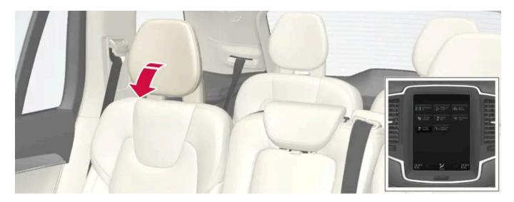
The outer head restraints can be retracted via the centre display's function view. You can lower the head restraints in ignition position 0.
