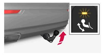
> The towbar extends out and down in an unlocked position - the indicator lamp flashes orange. The tow hook is ready to continue moving to the locked position.
