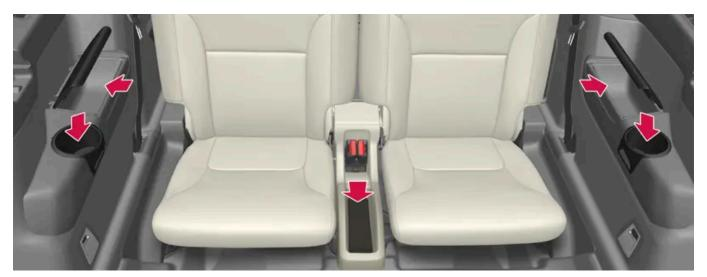
Storage compartment and cup holder in the side panel and storage space between the seats.
