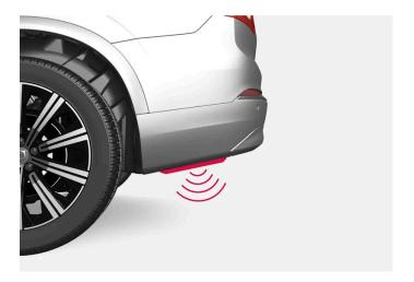
To activate opening or closing with a foot movement on a car equipped with skid plate, the kicking motion is made from the side of the car. One of the car's keys must be within range, approx. 1 metre (3 feet), for activation.
