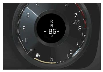
Gear shift indicator in the driver display<sup>[1]</sup>.
