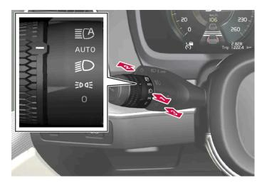
Steering wheel stalk switch with rotating ring.
