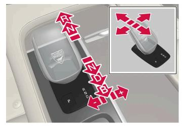
Overview of gear lever and gear positions.
