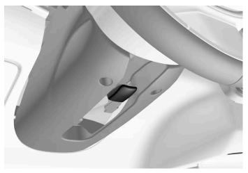
Lever for steering wheel adjustment.
