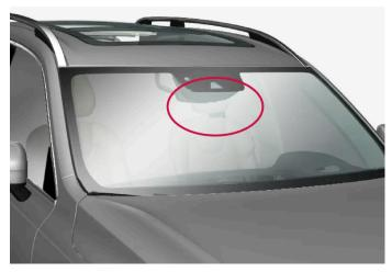
Location of front camera and radar unit
