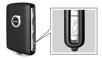
Unlocking the tailgate by pressing a button:
