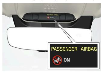
> A text message and a warning symbol in the roof console indicate that the airbag for the front passenger seat is activated.
