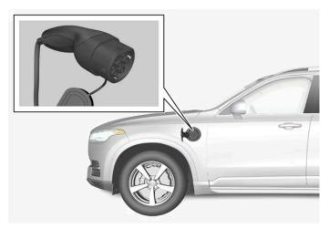
Charging cable handle and charging input socket.
