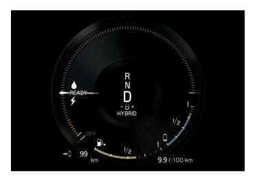
The hybrid gauge shows in different ways the relationship between how much power is being taken from the electric motor and how much power is available.
