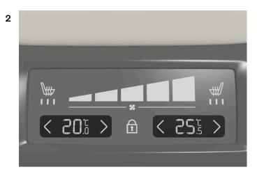
Temperature control on the climate panel at the rear of the tunnel console.
