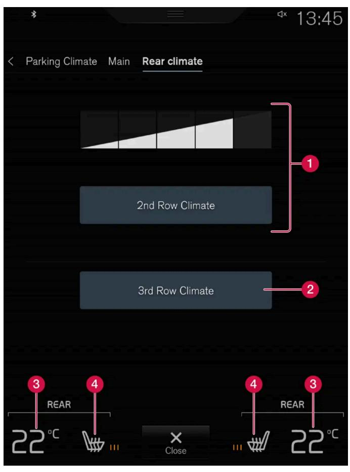
1 2nd row climate - Controls for climate functionality in the rear seat, second seat row. Fan controls for rear seat, second seat
