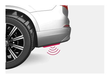
To activate opening or closing with a foot movement on a car equipped with skid plate, the kicking motion is made from the side of the car. One of the car's keys must be within range, approx. 1 metre (3 feet), for activation.
