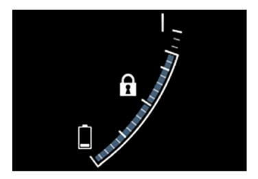
The symbol **f** is shown in the hybrid battery gauge when Hold is activated.
