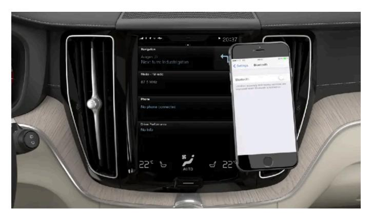
It is possible to have two Bluetooth devices connected at once, in which case one of them can only play back wirelessly. The most recently connected phone will automatically be connected to make calls, send/receive messages, play back media and provide an Internet connection [1]. It is possible to change what the phone is to be used for under **Bluetooth Devices** via the settings menu in the centre display's top view. Your mobile phone needs to be equipped with Bluetooth and support tethering.
