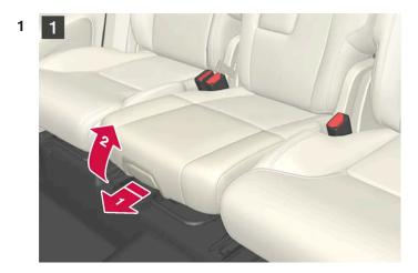
Pull the handle forwards and upwards to release the seat cushion.
