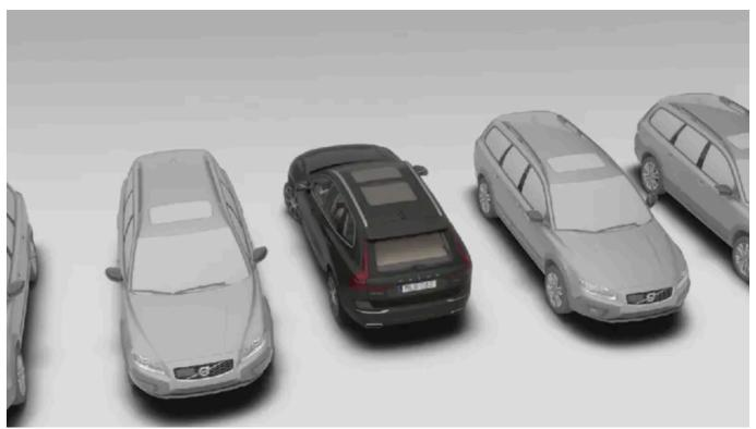
The function first checks if a space is large enough and if so then assists the driver to steer the car into the space.
