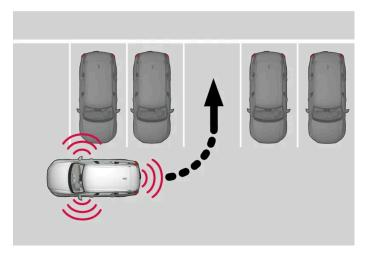
Principle for reversing into perpendicular parking.
