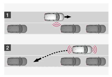
Principle for reversing into parallel parking.
