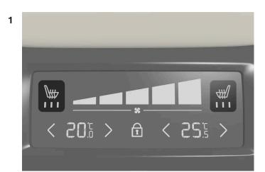
Seat heating indication and controls on the climate panel at the rear of the tunnel console.
