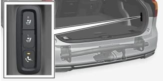
Open the tailgate. A button for extending/retracting the towbar is located on the right-hand side at the rear of the cargo area. An indicator lamp in the button must illuminate with a constant orange glow for the extension function to be active. 2 Press and release the button – extension might not start if the button is pressed for too long.
