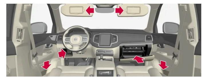
Storage compartment in the door panel and by the steering wheel, glovebox and sun visors.
