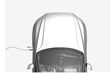
The hybrid battery is charged via a charging cable, but can be charged by gentle braking and engine braking in gear position B. The hybrid battery can also be charged by the car's engine. The car's starter battery is charged when the hybrid battery is charging.
