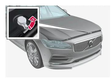
2 Turn the handle under the bonnet anticlockwise to release the catch and lift the bonnet.
