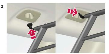
Guide one of the safety grille's hooks into the larger opening in the roof mounting (1). Grasp the grille near the hook and pull/slide it towards the smaller opening (2).
