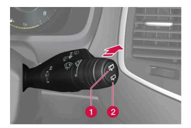
**2** Select 🖓 for continuous speed with the rear window wiper.
