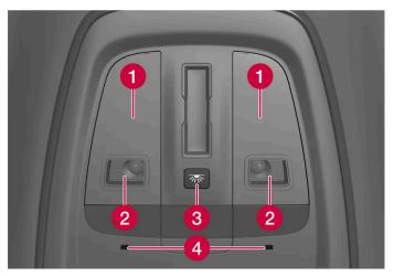
Lighting and controls in the roof console.
