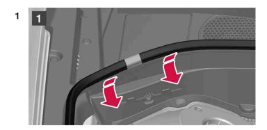
Lift off the rubber strip by pressing it inward in the engine compartment.
