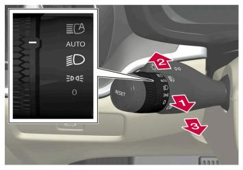
Steering wheel stalk switch with rotating ring.
