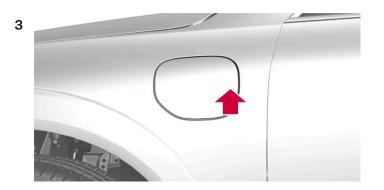
Press in the rear section of the cover to open the charging hatch and undo the cover for the charging input socket<sup>[2]</sup>.
