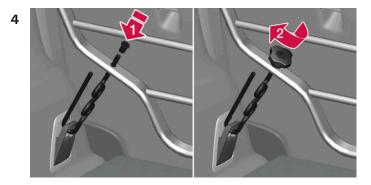
Hook the attaching brace's hook through the load securing eyelet at the cargo floor from underneath, and guide the threaded part through the cargo grille's lower attachment hole from underneath (1).
