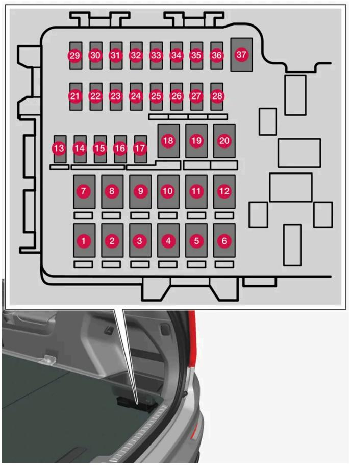
The content of this manual represents the status of the user manual at the time of printing and may not be completely valid in future instances. For more information, refer to the first page for the complete disclaimer note. 808 / 856 The central electrical unit is located under the storage compartment on the right-hand side.
