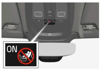
> A text message and a warning symbol in the roof console indicate that the airbag for the front passenger seat is activated.
