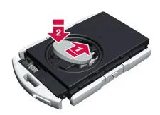
Install a new battery with the (+) side up. Avoid touching the key's battery contacts with your fingers.
