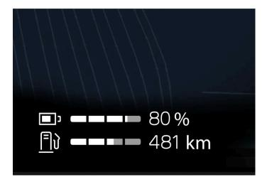
The battery gauge in the lower part of the driver display shows the State of Charge (SoC) for the battery as well as range to empty battery.
