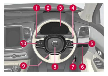
1 Position lamps, daytime running lights, dipped beam, main beam, direction indicators, rear fog lamp, resetting the trip meter
