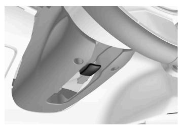
Lever for steering wheel adjustment.
