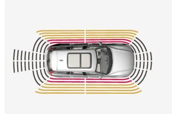
The warning signal pulses intensively at less than approx. 25 cm (0.8 foot) from an obstacle.
