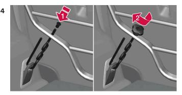
Hook the attaching brace's hook through the load securing eyelet at the cargo floor from underneath, and guide the threaded part through the cargo grille's lower attachment hole from underneath (1).
