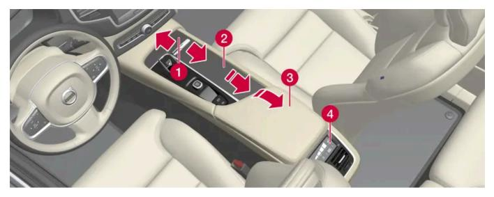
1 Storage compartment hatch \* and 12 V socket<sup>[1]</sup>. The hatch is opened/closed with a push on the handle.
