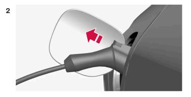
Unplug the charging cable from the car's charging input socket, refit the charging input socket's cover, and close the hatch.
