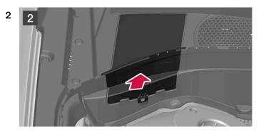
Detach the flap in the plastic cover by folding out the release catch and turning the flap upward.
