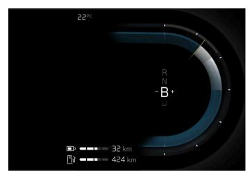
Gear shift indicator in the driver display.
