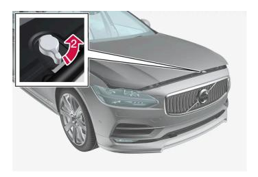
Turn the handle under the bonnet anticlockwise to release the catch and lift the bonnet.
