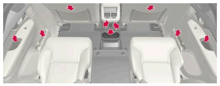
Storage compartment in the door panel, cup holder on the tunnel console's floor, in the centre seat backrest, storage pocket\* on the front seat backrest, as well as USB ports in the tunnel console.
