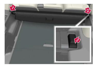
1 Insert one of the cargo cover's end pieces in the recess in the side panel in the cargo area.
