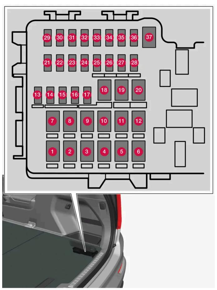
The central electrical unit is located under the storage compartment on the right-hand side.
