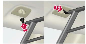
Guide one of the safety grille's hooks into the larger opening in the roof mounting (1).
