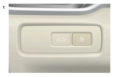
Press the button on the instrument panel.
