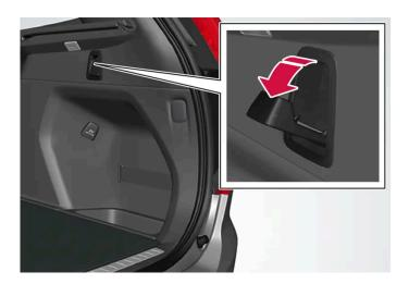
There are two extensible bag hooks in the side panels - one on each side of the cargo area.
