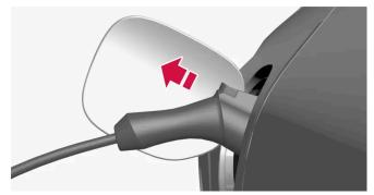
Unplug the charging cable from the car's charging input socket, refit the charging input socket's cover, and close the hatch.
