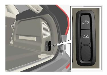
Use the buttons in the cargo area to regulate the height of the car's rear section and facilitate loading and unloading or when connecting or disconnecting a trailer.
