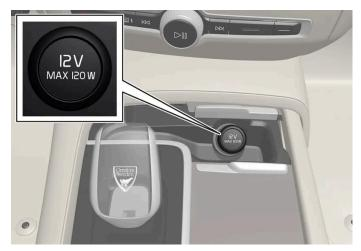
The tunnel console's front electrical socket for cars with wireless phone charger  $^{\star}$ .
