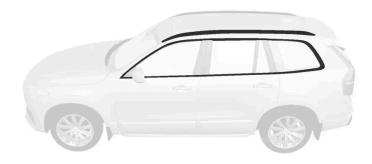
Parts that should be washed using a cleaning agent with a pH value between 3.5 and 11.5.
