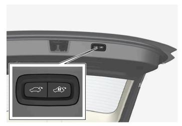
Location of the button/buttons on the underside of the tailgate.
