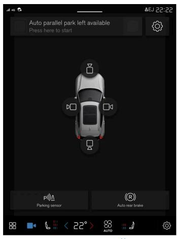
Camera view shows the park assist cameras (PAC<sup>[1]</sup>), which displays a composite 360° view and separate views for each of the four cameras: rear, front, left or right camera view.
