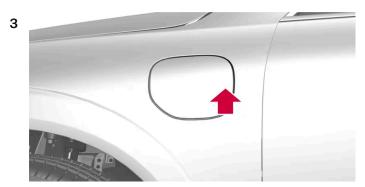
Press in the rear section of the cover to open the charging hatch and undo the cover for the charging input socket [2].
