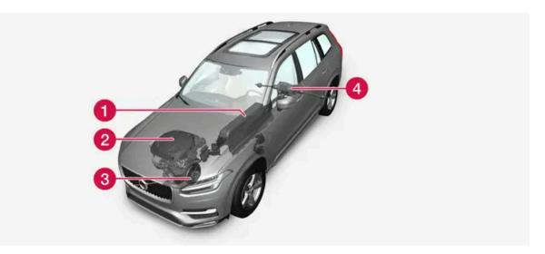
Hybrid battery - The function of the hybrid battery is to store energy. It receives energy when charging from the mains power circuit, during regenerative braking or from the high-voltage generator. It provides energy for electric operation as well as for temporarily operating the electric air conditioning during the preconditioning of the passenger compartment.
