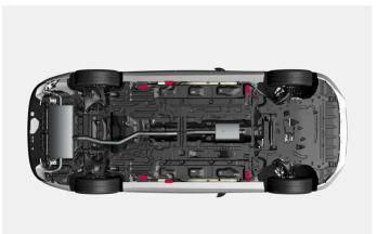
The car has outer lifting points for low level lifting, and inner lifting points for high level lifting, such as garage jack or lifting arms.
