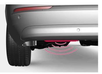
The sensor is located slightly to the left of the bumper.
