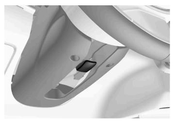
Lever for steering wheel adjustment.
