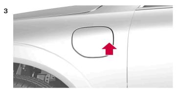
Press in the rear section of the cover to open the charging hatch and undo the cover for the charging input socket<sup>[2]</sup>.
