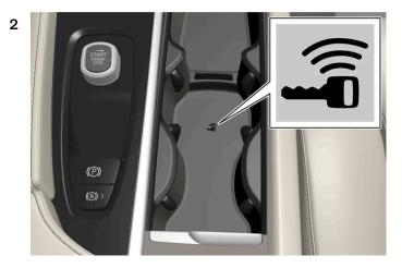
Place the key on the key symbol in the backup reader in the tunnel console's cup holder.
