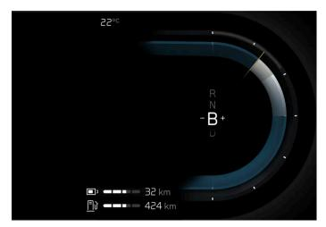
Gear shift indicator in the driver display.
