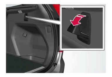
There are two extensible bag hooks in the side panels - one on each side of the cargo area.
