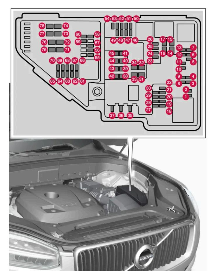
The content of this manual represents the status of the user manual at the time of printing and may not be completely valid in future instances. For more information, refer to the first page for the complete disclaimer note. 811 / 856 Special pliers are housed on the inside of the cover to facilitate replacement of tripped fuses.
