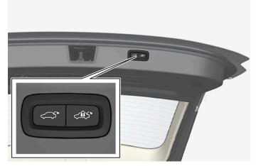
Location of the button/buttons on the underside of the tailgate.
