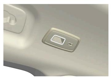
In cars with a panorama roof\*, the two lamp units are located on either side of the roof.<sup>[2]</sup>
