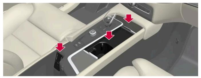
Storage spaces with cup holder, wireless phone charger\*, electrical socket, as well as USB ports in the tunnel console.
