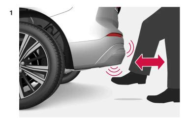
Make **one** forward kicking motion in the sensor area under the rear bumper. Then take a step back. The bumper must not be touched.
