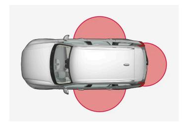
For keyless use, a key must be within a distance of approx. 1 to 1.5 metres (3 to 5 feet) from the car's doors or tailgate.
