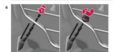
Hook the attaching brace's hook through the load securing eyelet at the cargo floor from underneath, and guide the threaded part through the cargo grille's lower attachment hole from underneath (1).
