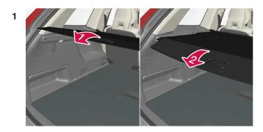
Grip the handle and pull out the cargo cover so that it slides over the side panels in the cargo area. Pull to the end position.
