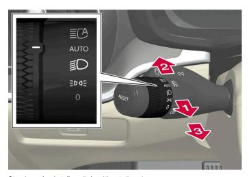
Steering wheel stalk switch with rotating ring.
