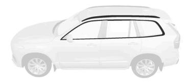
Parts that should be washed using a cleaning agent with a pH value between 3.5 and 11.5.
