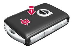
Turn the key and refit the front shell in the same way as for the rear.
