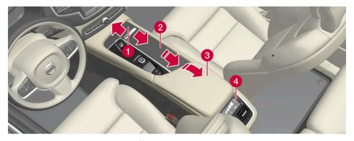
1 Storage compartment hatch\* and 12 V socket [1]. The hatch is opened/closed with a push on the handle.
