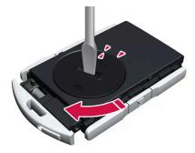
Refit the battery cover and turn clockwise to CLOSE position.
