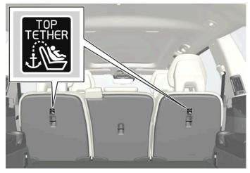
Five and seven seat variant: Mounting point locations for the second row of seats are indicated by symbols on the rear of the backrest.
