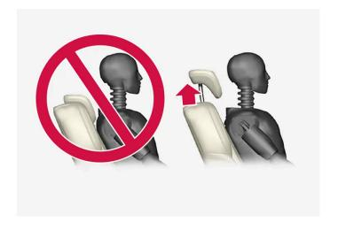
The centre seat's head restraint must be adjusted according to the passenger's height so that, if possible, the whole of the back of the head is covered. Slide it up manually as required.
