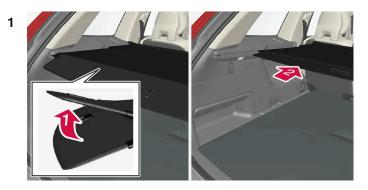
In the extended full-cover position - lightly push the handle part of the cargo cover upward, e.g. with an elbow.
