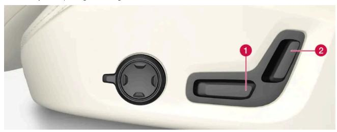
1 Move the passenger seat forward/backward by adjusting the control forward/backward.
