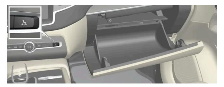
The glovebox is opened by pressing on the opening button in the centre console.
