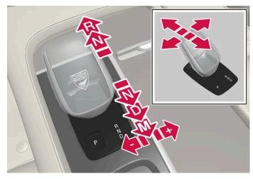
Overview of gear lever and gear positions.
