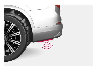
To activate opening or closing with a foot movement on a car equipped with skid plate, the kicking motion is made from the side of the car. One of the car's keys must be within range, approx. 1 metre (3 feet).
