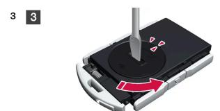
Turn the battery cover anticlockwise to OPEN position. Use a screwdriver or a coin, for example.
