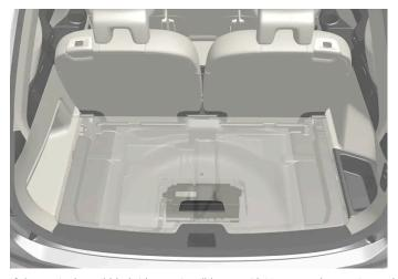
If the car is the mild hybrid type, it will have a 48 V support battery instead, located under the cargo area. The battery and the box covering it must only be handled by an authorised workshop.
