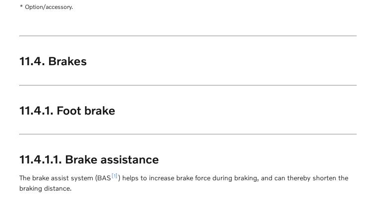
The system detects the way in which the driver brakes and increases brake force where necessary. The brake force can be boos-
