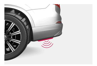
To activate opening or closing with a foot movement on a car equipped with skid plate, the kicking motion is made from the side of the car. One of the car's keys must be within range, approx. 1 metre (3 feet).
