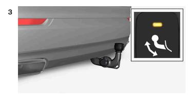
Move the towbar to its end position, where it is secured and locked in place - the indicator lamp illuminates with a constant orange glow.
