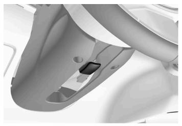
Lever for steering wheel adjustment.
