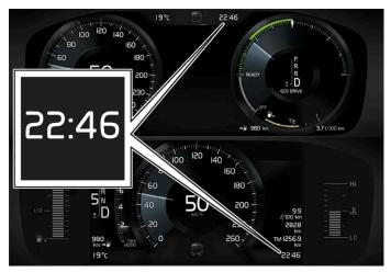
Clock location in the 12-inch\* and 8-inch driver display. The figure is schematic - parts may vary depending on car model.
