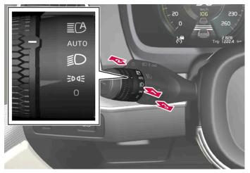
Steering wheel stalk switch with rotating ring.
