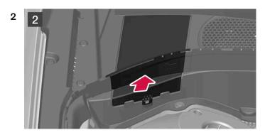
Detach the flap in the plastic cover by folding out the release catch and turning the flap upward.
