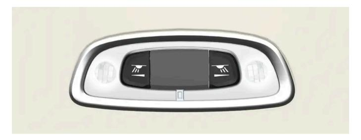
Reading lamps above the rear seat<sup>[1]</sup>.
