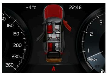
Graphics in the driver display with different types of warnings. The warning colour on the door and tailgate is dependent on the vehicle's speed.
