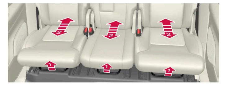
1 Lift the handle that is located under the seat.
