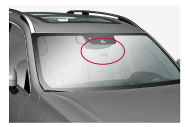
Location of front camera and radar unit
