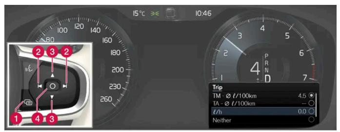
Open and navigate in the app menu<sup>[1]</sup> using the right-hand steering wheel keypad.
