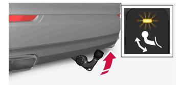
> The towbar extends out and down in an unlocked position - the indicator lamp flashes orange. The tow hook is ready to continue moving to the locked position.
