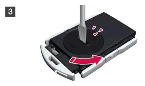
Turn the battery cover anticlockwise to OPEN position. Use a screwdriver or a coin, for example.
