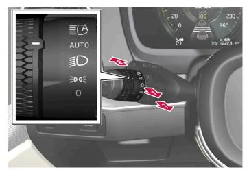
Steering wheel stalk switch with rotating ring.
