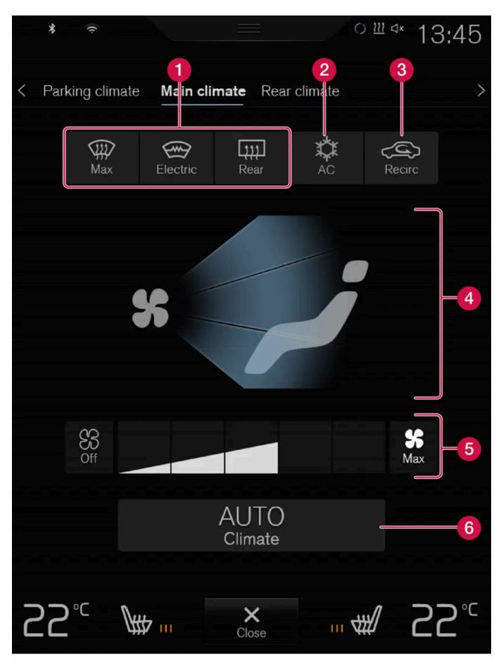
**<sup>1</sup>** Max, Electric, Rear - Controls for defrosting the windows and door mirrors.
