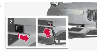
Front: Remove the cover – use the car's key or a small screwdriver in the socket to carefully prize off the cover.
