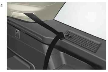
Hang up the locking tabs of the seatbelts for the third seat row on the designated hooks in the side panels.
