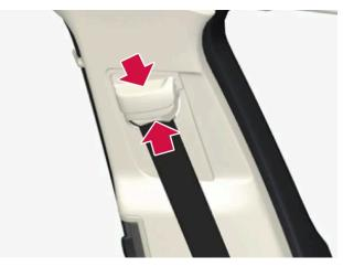
Press together the seat mounting and move the seatbelt up or down.
