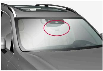
Location of front camera and radar unit
