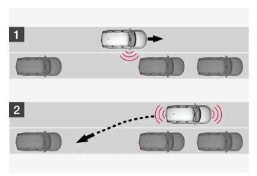
Principle for reversing into parallel parking.
