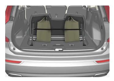
There are two bag hooks and an elastic strap<sup>[2]</sup> in the cover, which is part of the floor hatch in the cargo area. The strap can be fitted in four different positions.
