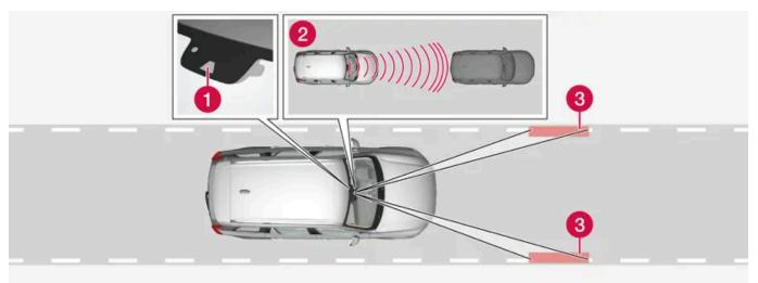
The camera and radar unit measures the distance to the vehicle ahead and detects side markings.
