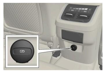
USB ports (type C) on rear of tunnel console for charging phones and tablets<sup>[1]</sup>, for example.
