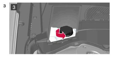
Screw off the cap and top up with coolant if necessary. The coolant level must lie between the MIN and MAX marks on the expansion tank.
