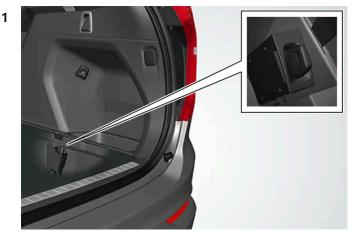
Fit a personal SIM card into the holder. Note that a **mini SIM** is required to fit the car's card reader.
