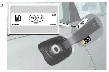
Choose fuel that is approved for use in the car in accordance with the identifier<sup>[1]</sup> on the inside of the fuel filler flap. See information on approved fuels and the identifier in the sections on "Petrol" and "Diesel" respectively.
