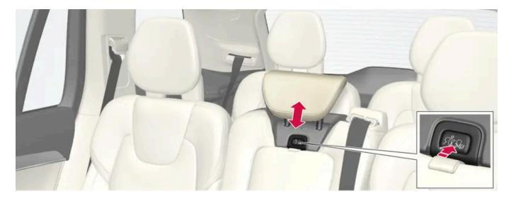
To lower the head restraint, the button (located in the centre between the backrest and head restraint, see illustration) must be pressed in while the head restraint is pressed down carefully.
