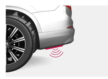
To activate opening or closing with a foot movement on a car equipped with skid plate, the kicking motion is made from the side of the car. One of the car's keys must be within range, approx. 1 metre (3 feet).
