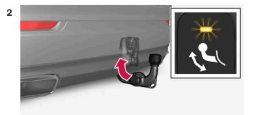
Lock the towbar by moving it back to its retracted position, where it is locked.
