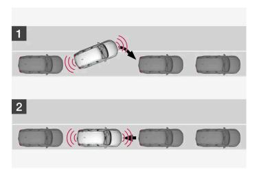
Principle for positioning during parallel parking.
