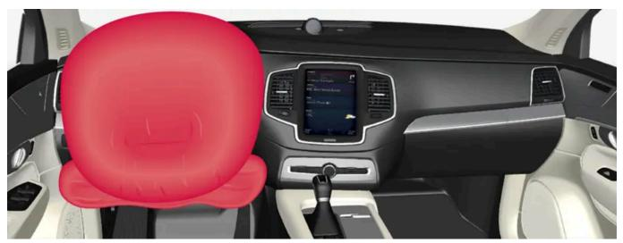
Steering wheel airbag and knee airbag on the driver's side in the front seat.
