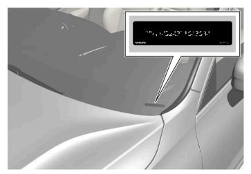
VIN is positioned in a similar place on all models.
