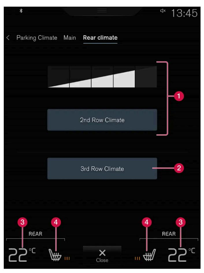
1 2nd row climate - Controls for climate functionality in the rear seat, second seat row. Fan controls for rear seat, second seat row.
