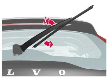
Lift the wiper arm from the window and pull the lower section of the blade to the right.
