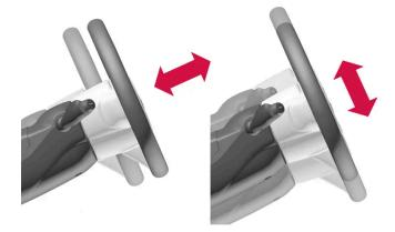
The steering wheel can be adjusted for height and for depth.
