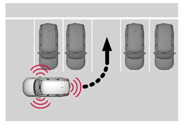
Principle for reversing into perpendicular parking.
