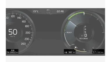
Examples of trip computer information in the 12-inch driver display\*. The figure is schematic - parts may vary depending on car model.
