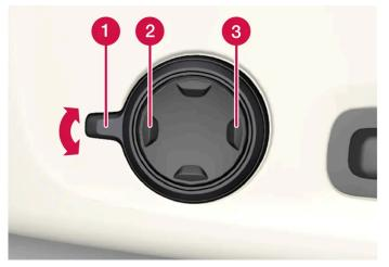
Multi-function button, located on the side of the seat base section.
