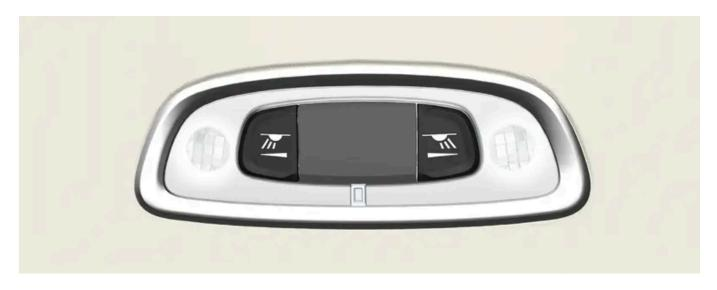
Reading lamps above the rear seat<sup>[1]</sup>.
