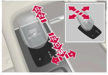
Overview of gear lever and gear positions.
