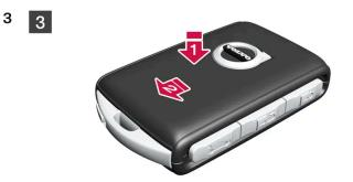
Refit the front shell in reverse order to how it was removed. Press in the shell until you hear a click, and then slide it the last few millimetres to its original position.
