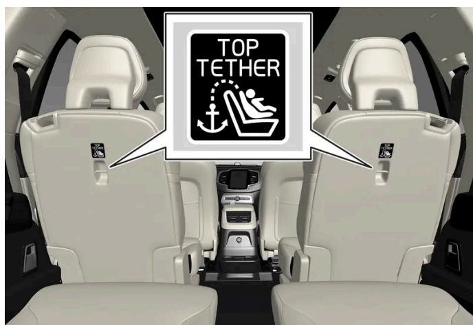
Six seat variant: Mounting point locations for the second row of seats are indicated by symbols on the rear of the backrest.
