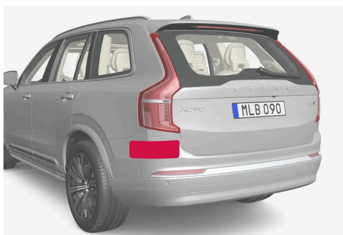
Location of rear radar units
