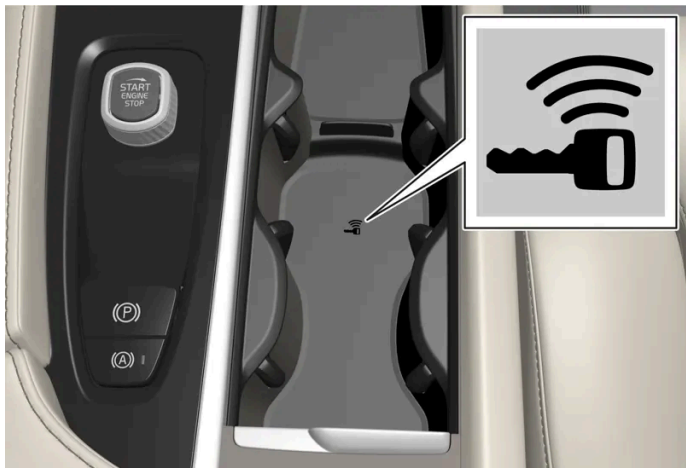
Backup reader's location in the tunnel console.
