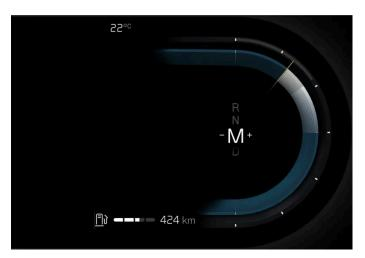
Gear shift indicator in the driver display.
