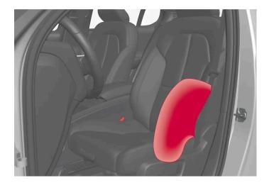
The near-side airbags are fitted in the outer backrest frames of the front seats and help to protect the driver and passengers in the front seat.
