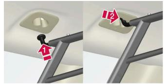
Guide one of the safety grille's hooks into the larger opening in the roof mounting (1).
