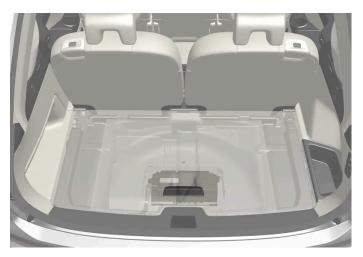
Cars of the mild hybrid type have a 48 V support battery located under the cargo area. The battery and the box around it must only be handled by an authorised workshop.
