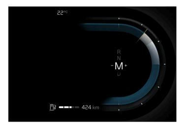
In M position, it is possible to change gear manually. The car engine-brakes when the accelerator pedal is released.
