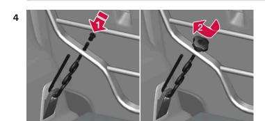
Hook the attaching brace's hook through the load securing eyelet at the cargo floor from underneath, and guide the threaded part through the cargo grille's lower attachment hole from underneath (1).
