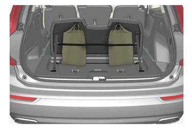
There are two bag hooks and an elastic strap [2] in the cover, which is part of the floor hatch in the cargo area. The strap can be fitted in four different positions.
