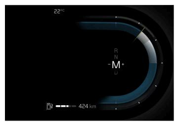
Gear shift indicator in the driver display.
