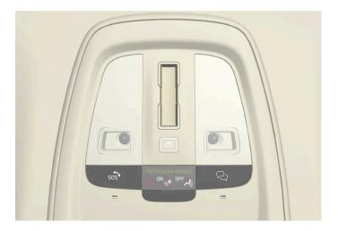
The panoramic roof and sun blind are operated with a control located in the roof.
