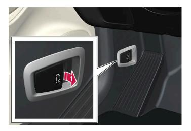
Pull the handle beside the pedals to release the bonnet from its fully closed position.
