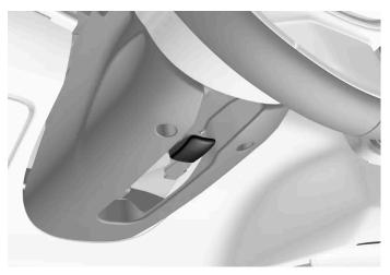
Lever for steering wheel adjustment.
