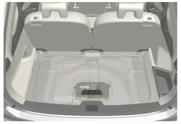
Cars of the mild hybrid type have a 48 V support battery located under the cargo area. The battery and the box around it must only be handled by an authorised workshop.
