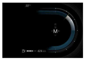
Gear shift indicator in the driver display.
