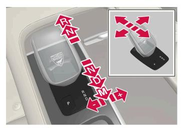
Overview of gear lever and gear positions.
