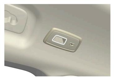
In cars with a panorama roof\*, the two lamp units are located on either side of the roof. [2]
