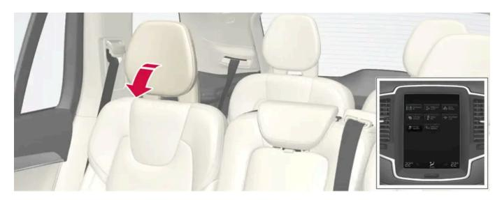
The outer head restraints can be retracted via the centre display's function view. You can lower the head restraints in ignition position 0.
