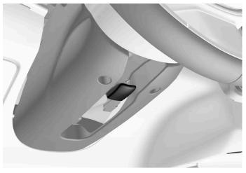
Lever for steering wheel adjustment.
