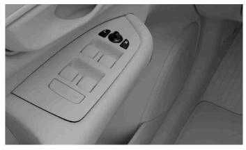
Controls for adjusting the wing mirrors
