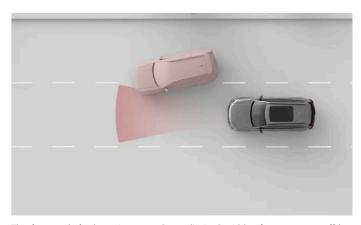
The front radar's detection zone has a limited width. If you get cut off by another vehicle, detection can occur relatively late causing a sudden response by your car.
