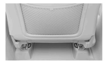
The lower tether anchorage points can be found at the back of the floor rails of the front seats.
