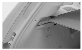
Slide the ends of the load cover screen into the upper grooves of the side panels.
