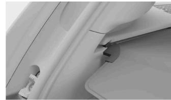
Guide the ends of the load cover into the locked position in the grooves.
