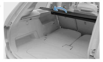
Pull the load cover screen by the handle over the boot's side panels.
