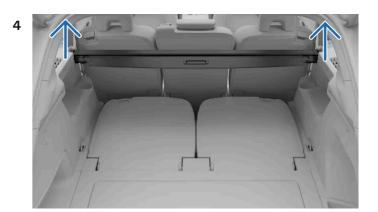
Lift the load cover completely from the indentations at the back of the boot to remove it.
