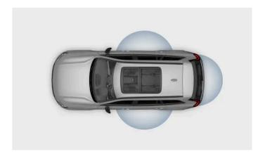
The standard key's buttons have a long range of detection. If your car doesn't respond to a button being pressed, try moving closer.
