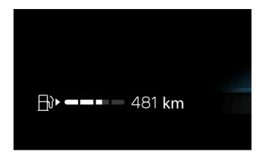
Your range is primarily related to the amount of fuel left in your car's tank and your driving practices but external conditions can also be a factor. The fuel meter and expected range are displayed in the driver display.
