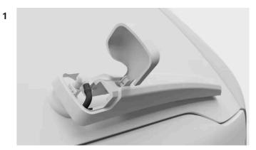
Find the plastic cover where the wiper arm attaches to the car. Loosen the side of the cover closest to you first and then the side furthest away from you. Lift the plastic cover up fully. This will give you access to the hose connector.
