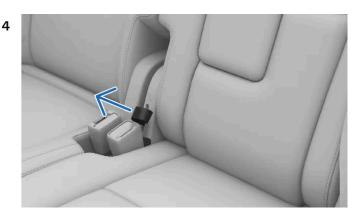
Pull and hold the strap on the side of the seat to unlock backrest movement.
