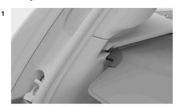
Lift and pull the end of the load cover screen by the handle to unlock it.
