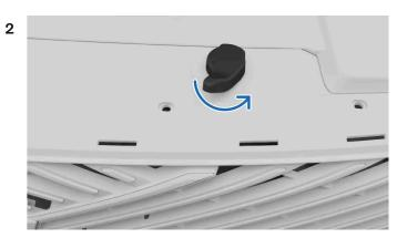
Locate the second lever below the front edge of the bonnet and rotate it anticlockwise.
