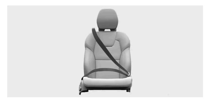
The seatbelt locks itself to act as a safety restraint under certain conditions, such as sudden and forceful pulling of the belt, if the car is driven aggressively and if the car is on a steep incline.
