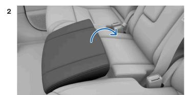
Using one hand on the front of the child seat and one on the rear, guide the child seat upwards and back all the way to the backrest of the seat.
