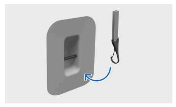
Fastening tether to top tether anchorage point
