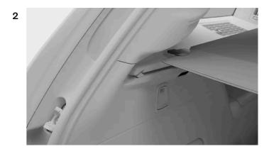
Lift the ends of the load cover screen through the bend. Keep hold of the handle and guide the load cover screen out of the upper grooves. This allows the screen to automatically retract.
