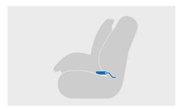
Child restraint installed using ISOFIX
