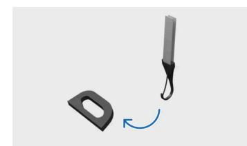
Fastening tether to lower tether anchorage point
