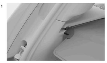
Lift and pull the end of the load cover screen by the handle to unlock it.
