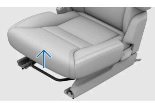
Grasp and pull the handle under the seat cushion upwards.
