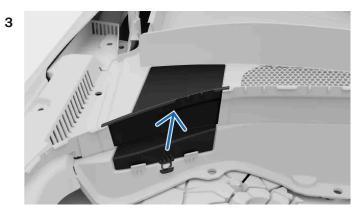
Open the hatch lock and lift the hatch upwards to release it.
