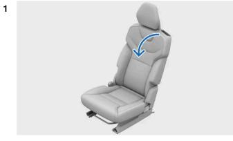
Pull the handle on the top of the outer seat backrest.
