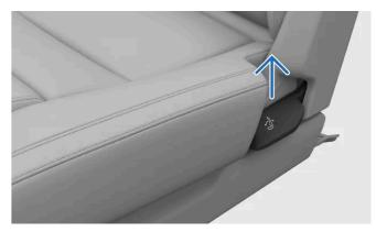
Pull the handle on the side of the seat upwards.
