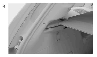
Slide the ends of the load cover screen into the upper grooves of the side panels.
