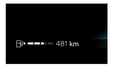
The driver display shows the fuel meter at all times.
