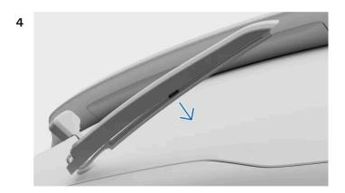
Pull the blade down until it loosens and comes away from the wiper arm.
