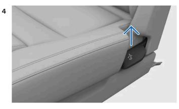
Pull and hold the handle on the side of the seat upwards to unlock backrest movement.
