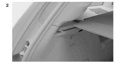
Lift the ends of the load cover screen through the bend. Keep hold of the handle and guide the load cover screen out of the upper grooves. This allows the screen to automatically retract.
