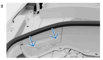
The coolant container is located in the upper-left corner of the engine compartment, underneath a panel hatch. Pull the rubber seal towards the engine compartment to access the hatch.
