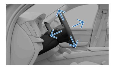
Adjusting the steering wheel position is fundamental to your driving posture, allowing you better comfort and control of the car.
