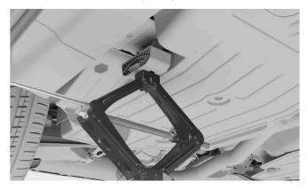
**9** Raise the car to an appropriate height. Do not raise it higher than what's necessary for the work you're doing.
