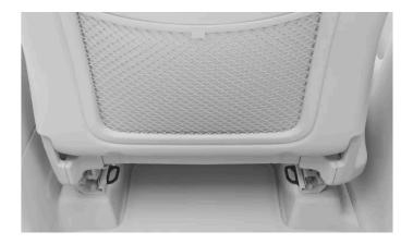
The lower tether anchorage points can be found at the back of the floor rails of the front seats.
