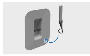
Fastening tether to top tether anchorage point
