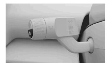
You control the rear windshield wiper by using the lower button on the left-hand steering wheel stalk.
