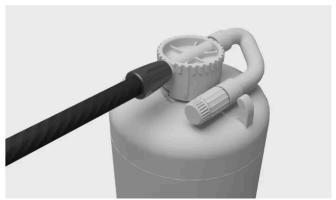
Screw the air hose to the sealing fluid bottle. There's a place for it opposite the sealing fluid hose.
