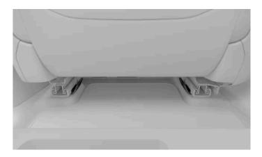
The lower tether attachment points for the rear seats can be found at the back of the floor rails of the seats in front. (i) Note Manufacturer's instructions When using attachment points, always follow the instructions from the manufacturer of the child restraint.
