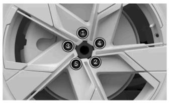
Tighten the wheel fasteners crosswise.
