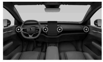
The positions of the adjustable air vents.
