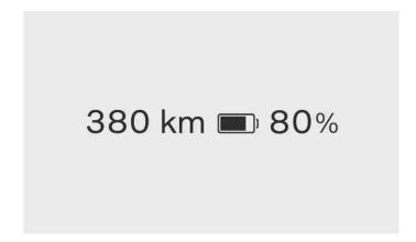
The battery meter is shown in the driver information area at all times. The battery icon's color changes depending on the level of charge remaining on the battery.
