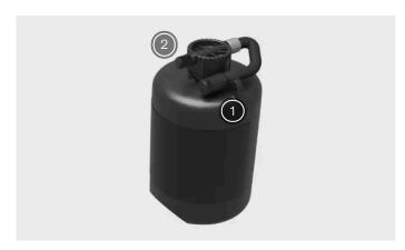
Overview of the temporary puncture repair kit sealing fluid bottle
