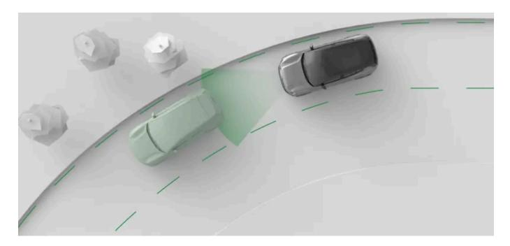
Pilot Assist actively guides your driving in a number of ways. When driving with Pilot Assist, you select the target speed. The vehicle then manages acceleration and braking to meet that target while also adapting to surrounding traffic.
