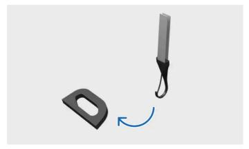
Fastening tether to lower tether attachment point
