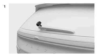
Find the plastic cover where the wiper arm attaches to the vehicle. Loosen the side of the cover closest to you first and then the side furthest away from you. Lift the plastic cover all the way. This will give you access to the hose connector.
