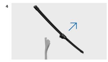
Remove the wiper blade from the wiper arm.
