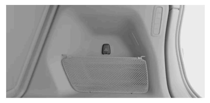
The 12 V electrical socket is on the right-hand side in the trunk.
