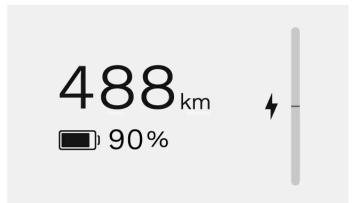
Your range is primarily related to your vehicle's battery level and your driving practices, but external conditions can also be a factor. The battery level and expected range are displayed in the instrument panel. The expected range is calculated based on your driving pattern, both current and historical.
