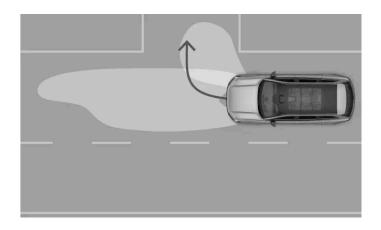
The cornering lights illuminate the area close to the vehicle to give you better visibility when turning.
