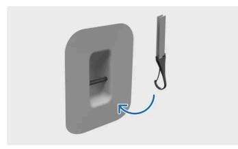
Fastening tether to top tether attachment point
