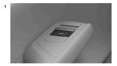
Press the window symbol *C* to switch between controlling the front and rear windows. The current window selection is indicated by the lights next to the symbol.
