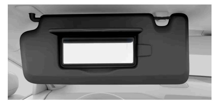
The visors can be folded down and angled to the side when necessary. With the sun visor angled to the side, you can also extend the rod holding the sun visor for better positioning.
