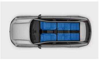
Your vehicle's passenger compartment is divided into different climate zones All zones are directly synced to the driver's preferred climate settings by default. However, the rear zones can have their own individual temperature setting.
