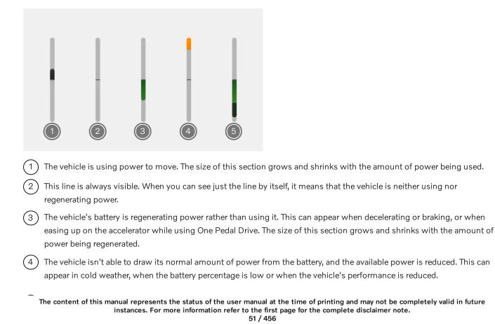
5) The friction brakes are in use. You might see this section appear when the disc brakes are engaged or if the battery is full and can't store any more power. The more you apply the friction brakes, the larger the section becomes.
