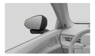
When the vehicle detects traffic that is about to pass close to the sides, a light appears in the door mirror. If you begin to open the door on the side of the detected traffic, the alert intensifies. An audible alert can occur along with the visual alerts, depending on how urgent the warning is.
