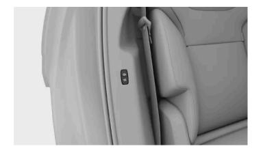
When a rear door is open, you can find the folding buttons in the door frame. There is one identical set of buttons on each side of the vehicle. These locations can be useful if you plan to fold both the second- and third-row seats .
