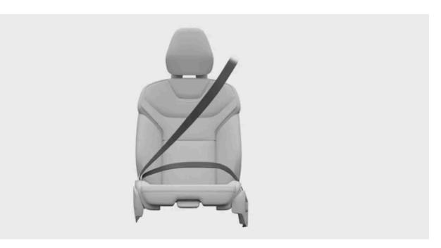
The seat belt locks itself to act as a safety restraint under certain conditions, such as sudden and forceful pulling of the belt, if the vehicle is driven aggressively and if the vehicle is on a steep incline.
