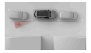
Door opening alerts are designed to warn you of passing traffic so that you don't open a door in its path. These alerts can be provided when the vehicle is stationary or moving very slowly<sup>[1]</sup>.
