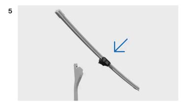
Make sure that the blade for the driver side is longer than the blade for the passenger side. Whilst keeping the wiper blade horizontal, slide the wiper blade onto the wiper arm. Ensure that the pin on the wiper arm goes into the hole on the wiper blade.
