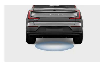
The sensor detects movement under the rear bumper. Any detected movement unlocks the trunk.
