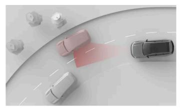
On a curve, the vehicle ahead may slip out of the detection zone. Vehicles in the adjacent lane may also enter the zone, affecting your vehicle's perception of the distance to traffic ahead.
