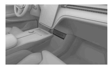
There are two USB ports<sup>[1]</sup> under the center display.
