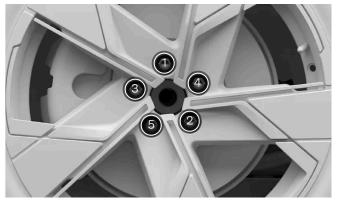
Tighten the wheel fasteners crosswise.
