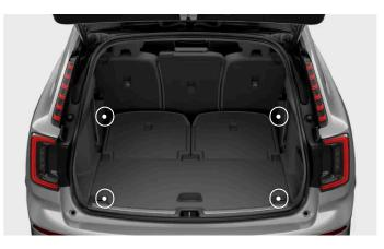
Load-retaining eyelets are located in the four corners of the trunk. You can use the load-retaining eyelets to attach straps and secure cargo in the trunk.
