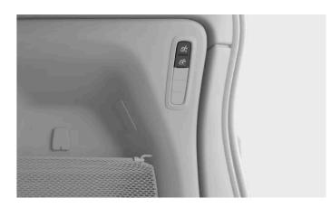
On the right-hand side in the trunk, there is a button panel. The top two buttons, one for each seat, can be used to fold and raise the third-row seats. This location can be useful if you need more room for stowing while using the trunk.
