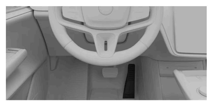
Braking behavior changes through the use of the accelerator pedal. When you press the accelerator, the vehicle accelerates normally, but releasing the pedal engages braking. The more you ease up on the pedal, the more braking action you get. By releasing the accelerator completely, you will eventually bring your vehicle to a full stop.
