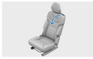
Pull the handle on the top of the outer seat backrest.
