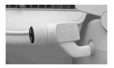
• Press and hold the button on the left-hand steering wheel stalk for the washers you want to activate. The front washers
