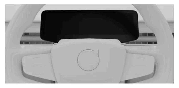
The instrument panel is located in front of the driver, behind the steering wheel. Its position changes along with the steering wheel when you adjust it to your preferred driving posture.
