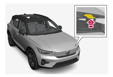
Move the handle under the hood upwards to release the catch and lift the hood.
