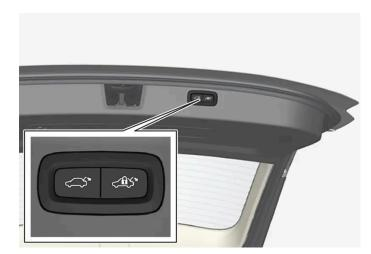
Location of button(s) on underside of tailgate.
