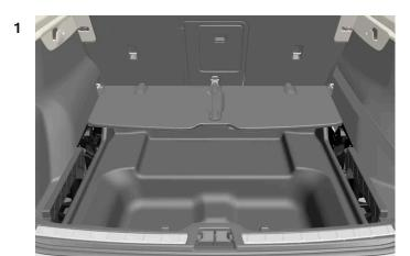
Fold the cargo compartment floor forward to position the parcel shelf with its top facing down and its rear part facing forward.
